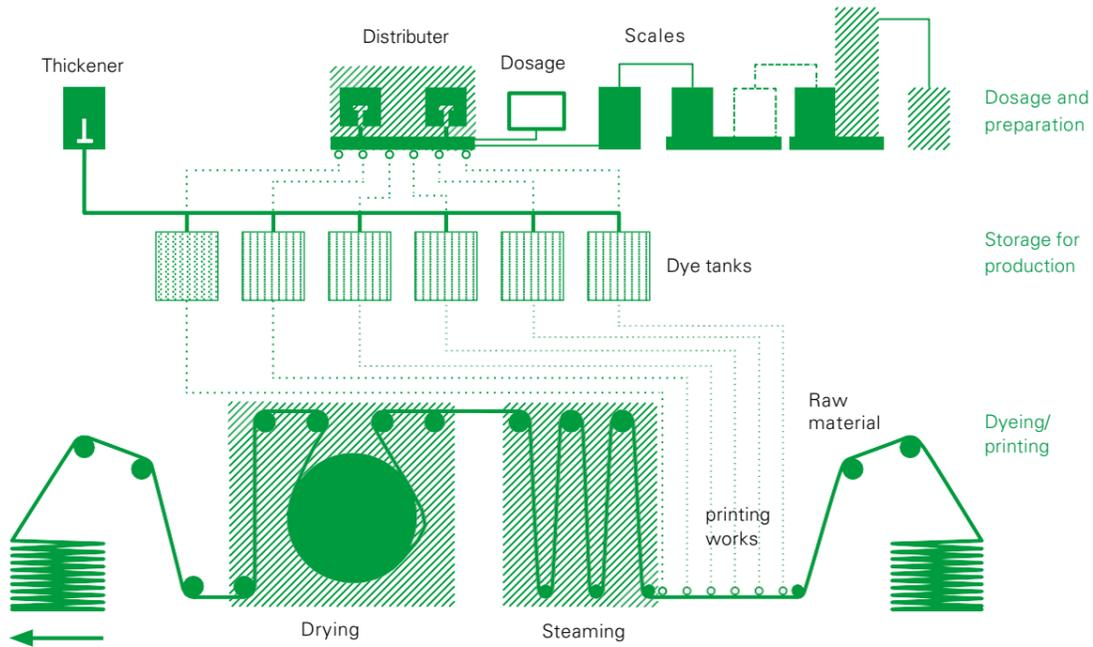
DYE DOSAGE AND BATCH PREPARATION STATION
